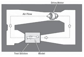
can be studied in different ways. Smoke or dye can be placed in the air and can be seen as it moves. Threads can be attached to the object to show how the air is moving. Special instruments are often used to measure the force of the air on the object.
